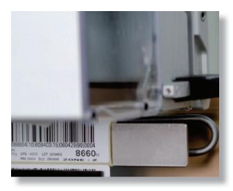
The 2000 Series systems, equipped with a tamp applicator, print the 23 figures in the EAN 128 code on each box at the rate of 25 boxes per minute.
